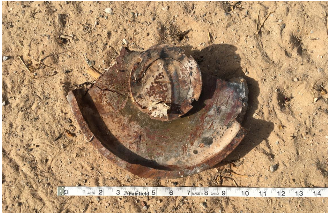
The intact baseplate of an unguided French 250kg SAMP aircraft bomb, recovered by Amnesty International investigators from the crater left by the strike on the home of the Qreira family. ©Amnesty International
