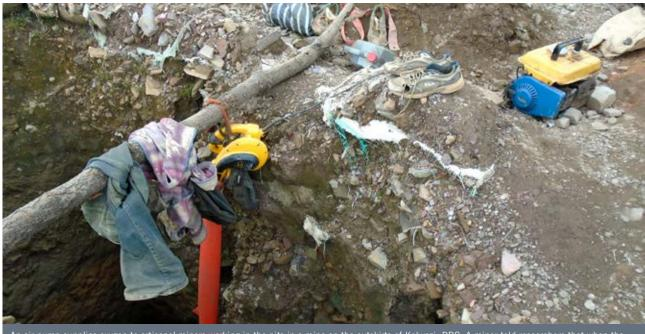
An air pump supplies oxygen to artisanal miners working in the pits in a mine on the outskirts of Kolwezi, DRC. A miner told researchers that when the generators run out of fuel, they cannot breathe and need to climb out as fast as possible, May 2015. © Amnesty International and Afrewatch
