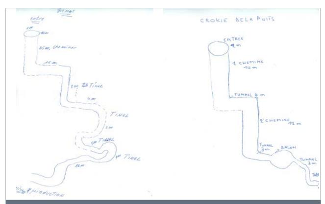
Diagrams drawn by artisanal miners to show the layout and depth of their mine. The miners dig the tunnels using hand tools, following the seam of cobalt ore as it winds and descends down through the earth. The tunnels often go beyond the maximum depth of 30 metres stipulated by the DRC's Mining
