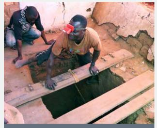
Miners climb out of a mine shaft by placing their hands and feet in holes carved out of the sides of the pit shaft. They use a rope attached to a beam stretched over the mouth of the pit as support. Sometimes the rope cuts and miners fall, a miner told researchers, May 2015
