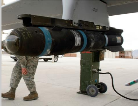
A Hellfire missile attached to an MQ-1B Predator. © Ethan Miller for Getty Images
