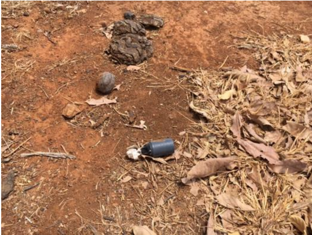
This image is a sub-munition from a cluster munition and bears a strong resemblance to the M20G sub-munition of Greek manufacture, which are fired using 107mm artillery shells. Karkarai, Um Dorrein, April 2016 © Transformedia CiC
