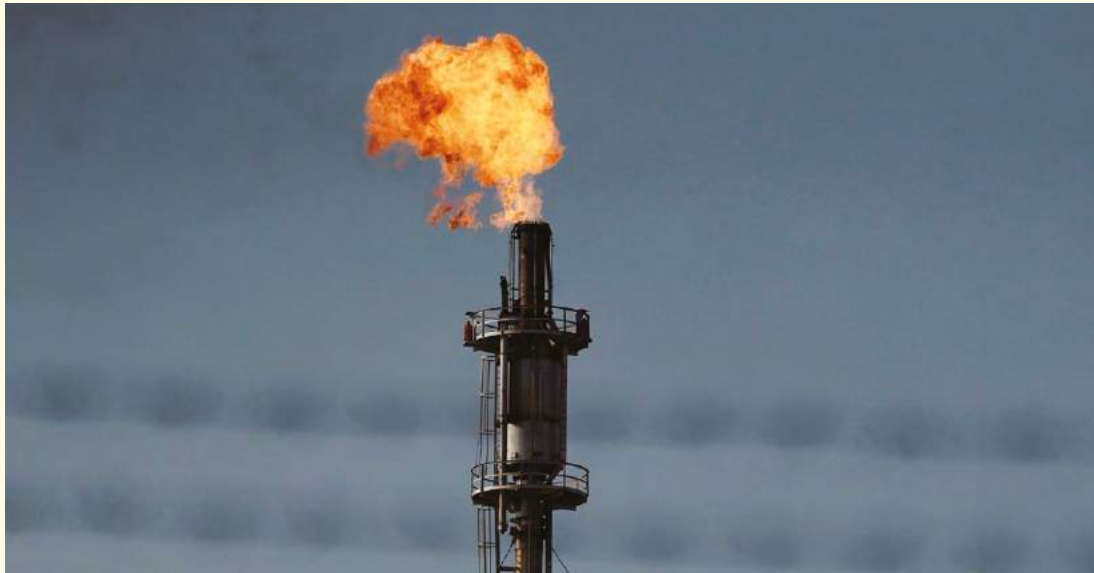
Flames from a flare stack. Flaring is used by petrochemical plants and refineries to burn off excess gas. © 2019 Getty Images/ Bloomberg Creative (Photographer: Dimas Ardian)
