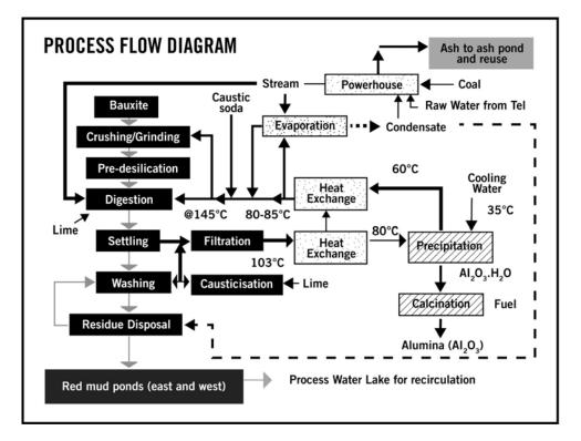
Flowchart 1: Process Flow Diagram of the Lanjigarh refinery (source: OSPCB Inspection Report on Vedanta Aluminium, 2-4 November 2007)
