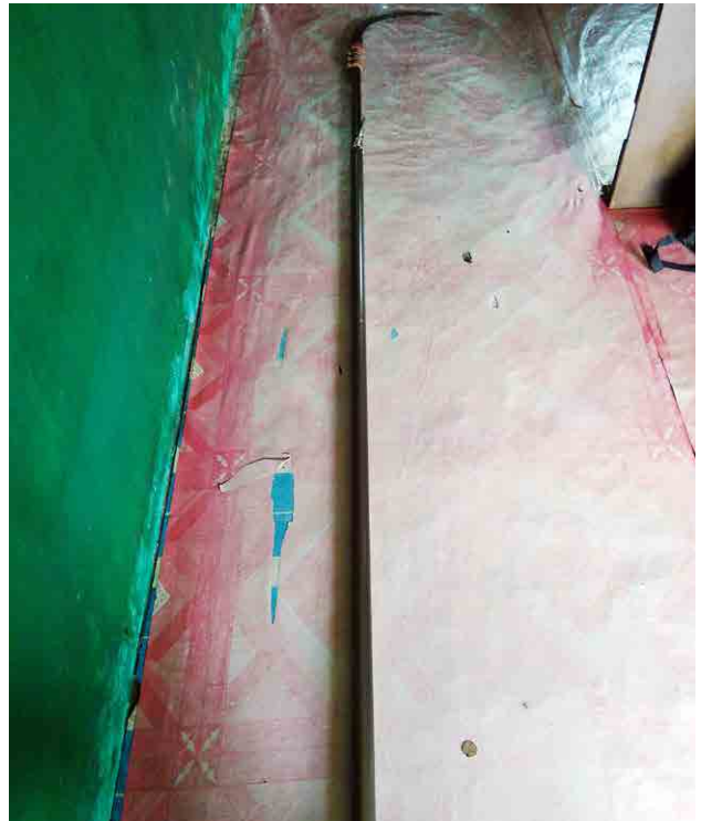
Egrek - long steel poles with a sickle at the end, which can weigh around 12kgs, that harvesters use to cut palm fruit bunches from tall trees. © Private
