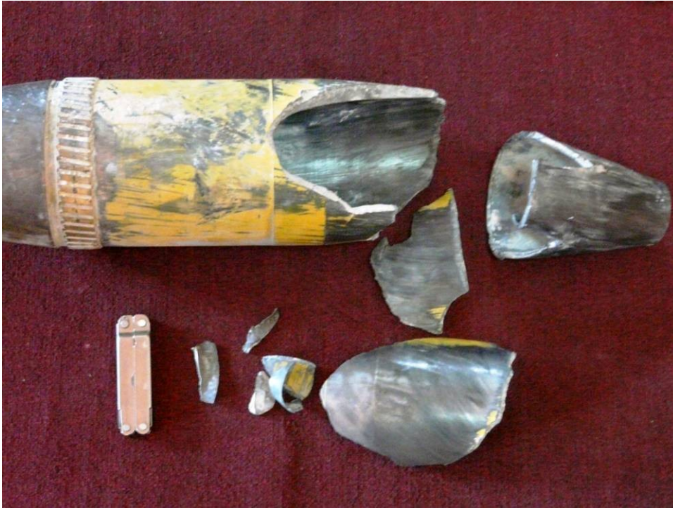
An artillery carrier shell which ejects a canister for illumination © Amnesty International
